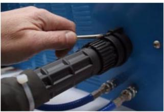
Note that a sealing ring is located in the base of the torch connector socket to form an air seal with the centre power pin. Care should be taken to ensure that this seal is not displaced and that the end of the pin is not damaged when the torch plug is removed.
