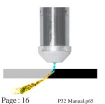
MAXIMUM CUTTING SPEED Drag back of the arc is around 45°, but cut quality will deteriorate.
