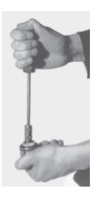
3. Unscrew the Nozzle with the special tool supplied. (See illustration left).
