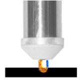
If the torch is pivoted about the nozzle there is a risk of material being blown back onto the nozzle which will cause damage to the nozzle or even to the torch itself.
