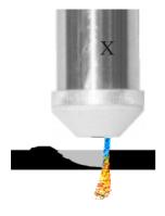
As piercing completes, the nozzle can be brought to vertical and cutting can continue.
