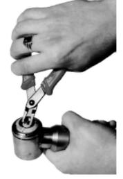
4. Check the condition of the Electrode Assembly. If it is to be removed, grip the Electrode Assembly with the special Electrode Pliers provided, and pull firmly out from the torch body. (See illustration right).
