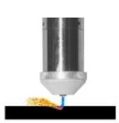
CUTTING TOO FAST Arc fails to pierce the material. Blow back of dross will damage the nozzle.
