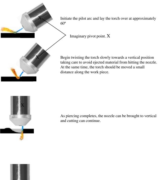
If the torch is pivoted about the nozzle there is a risk of material being blown back onto the nozzle which will cause damage to the nozzle or even to the torch itself.
