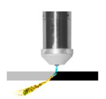
MAXIMUM CUTTING SPEED Drag back of the arc is around 45°, but cut quality will deteriorate.
