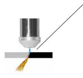
Under normal cutting conditions the torch is designed to operate with a STAND OFF of about 6 mm. This is the distance between the end of the nozzle and the work piece.
