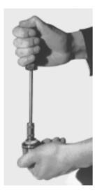
3. Unscrew the Nozzle with the special tool supplied. (See illustration left).
